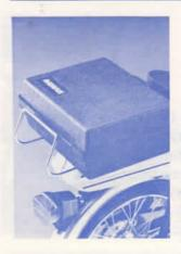
AC 117—Rack Extender—Designed for 1978 single seat models chrome plated, solid steel, carries baskets, saddle bags, or carry-all.
